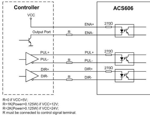
Figure 2: Connections to controller with differential outputs
