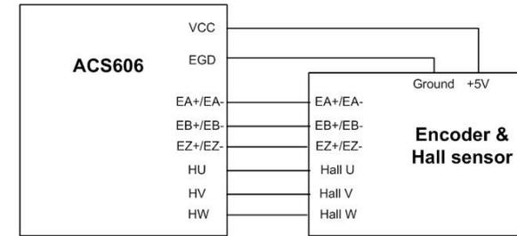
Figure 7: The ACS606 supplies the encoder directly
