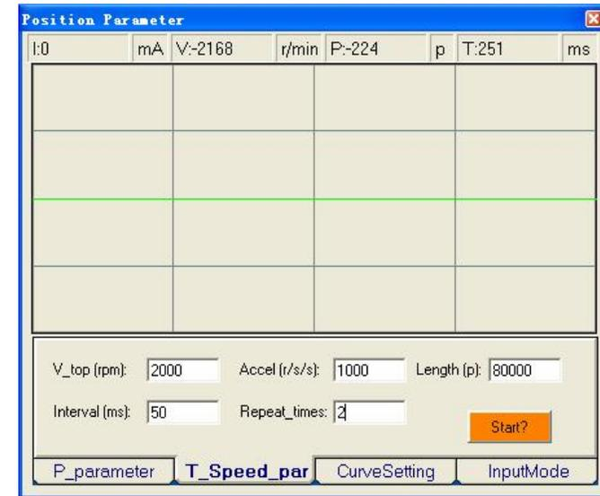
Figure 31: Self-test motion settings for the tuning
