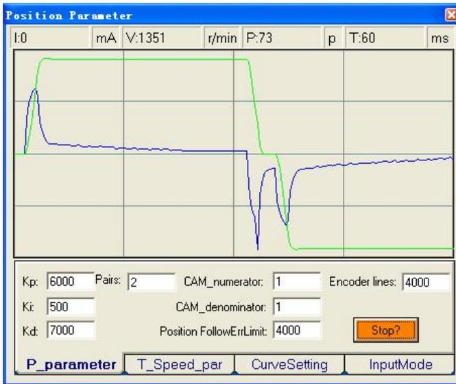
Figure 38: Position following error curve and velocity curve (Kp=6000, Ki=500 and Kd=7000)
