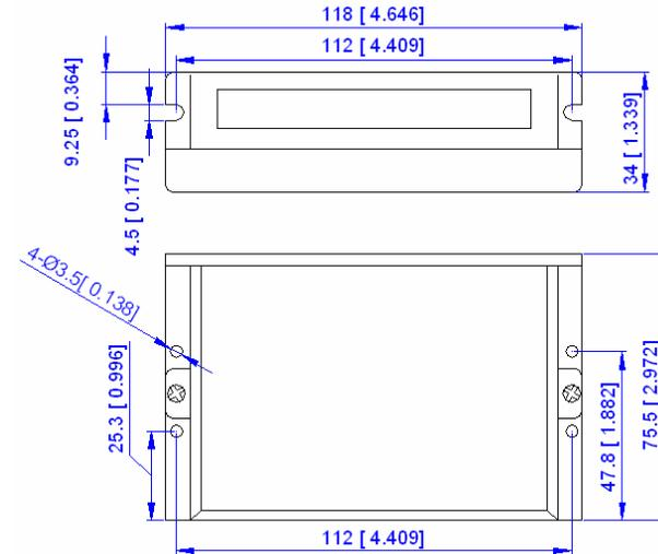
Figure 1: Mechanical specifications
