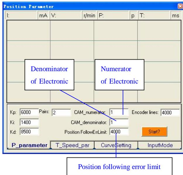
Figure 50: Electronic gear and position following error setting
