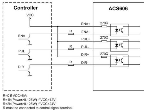
Figure 3: connections to controller with Common-Anode outputs
