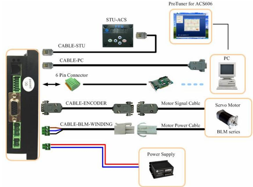
Figure 53: ACS606 accessories and connections with extended cable
