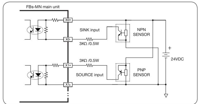
Wiring of 24VDC single-end SINK input
