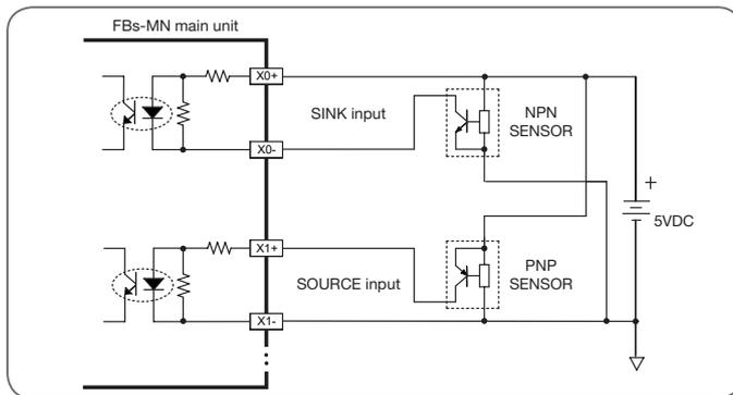
Wiring of 5VDC differential input to 24VDC single-end
