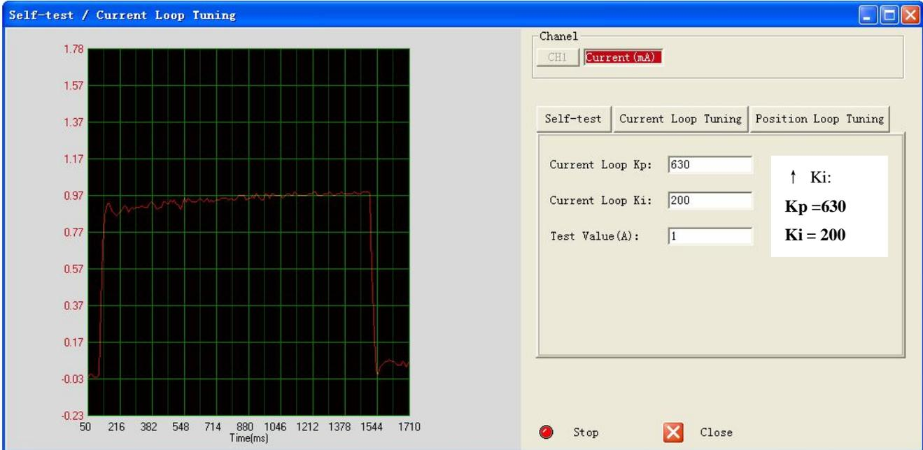
**Step 5:** The current loop tuning is basically finished. You can continue to adjust Kp and Ki for better performance. Now the updated Kp and Ki is just stored in the driver's RAM. They will be lost when we power off the driver. Don't forget to click the **Save to Drive** icon to store the changed value to the drive's EEPROM. See below.
