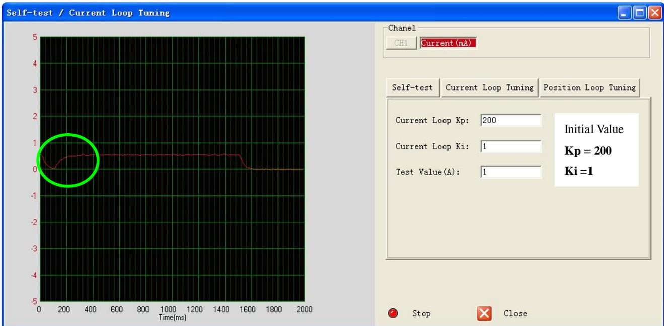
**Step 2:** Click the **Start** button and the plot window shows the step response of the current test. As the red curve increases from 0 to target slowly, it indicates that a large **Kp** needs to be introduced.
