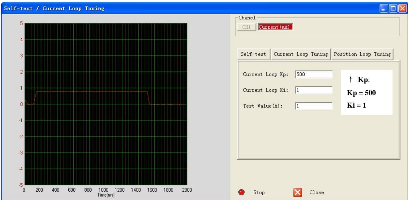
**Step 3:** Give **Kp** 600, 700 and click **Manual Tuning**, respectively. The red curve is changing faster. Over-shoot is obvious when increase **Kp** to 700. It indicates that you need to stop increasing Kp and back off. So we decrease Kp to 650 until the actual value is exactly over the target value.
