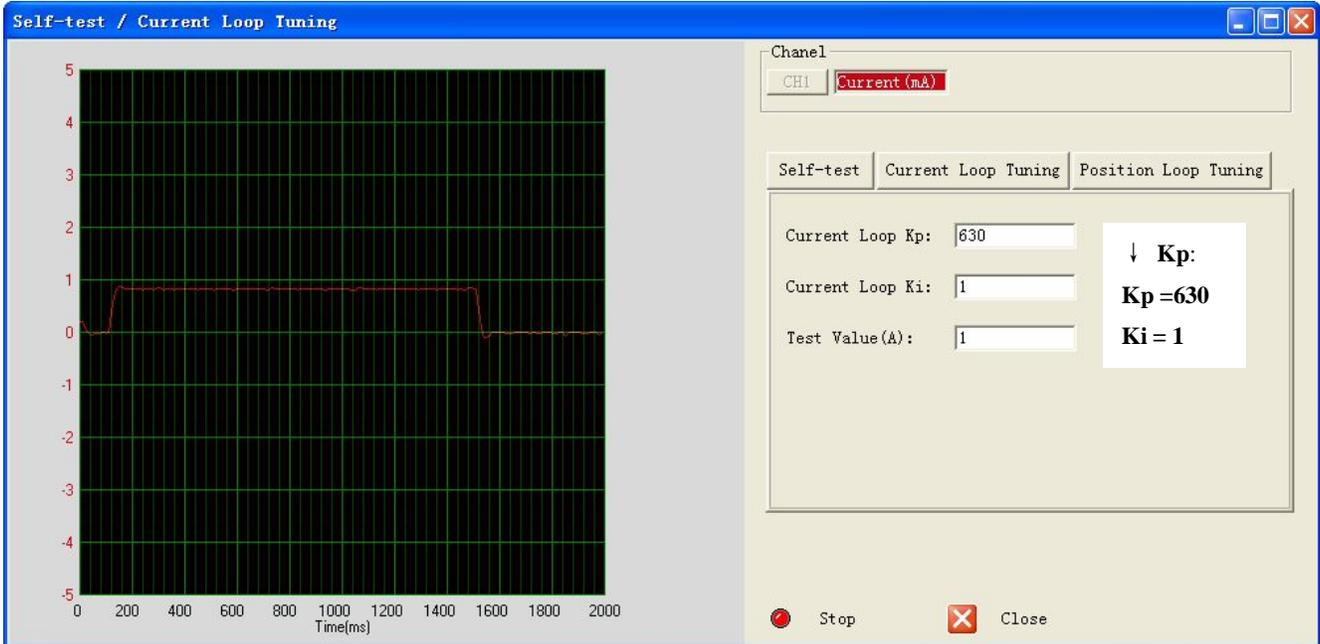
**Step 4:** Now the **Kp** is relatively good enough. But there is still error between the command current and the target current. So we need to introduce **Ki** to reduce the steady error at the constant part. It follows the same procedure as **Kp**. High **Ki** causes big vibration, system lag and makes the performance worse. The following figures show how to tune the integral gain.
