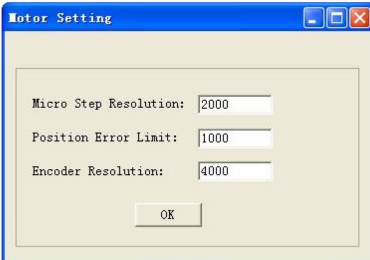
High resolution Micro Step makes the motor move more smoothly. Low Micro Step resolution reduces the high frequency requirement to the controller. If the application requires small position following error, reduce the **Position Error Limit**. The encoder resolution is 4 × actual encoder resolution.
