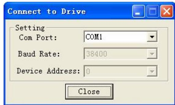
**Connect to Drive** window appears every time you open ProTuner. You can also open it by clicking **System->Connect To Drive** when the software is open. . Select the serial port number and click on the **Open** button. The software will try to connect to the drive and read the settings. It may take several minutes. Please wait.
