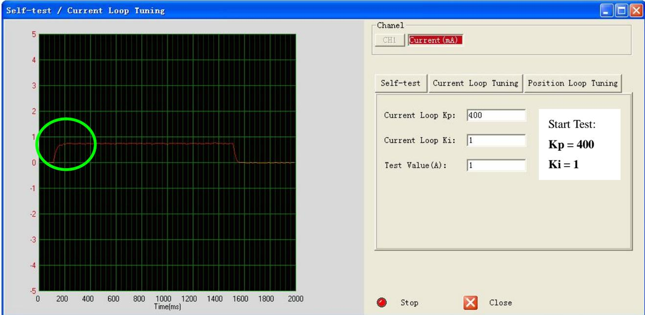
**Step 3:** Increase **Kp** to 500 and click **Start**. The red curve change faster from 0 to the target..
