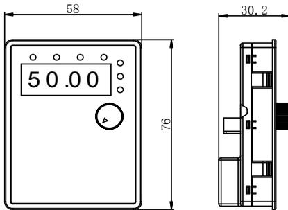
Keypad dimension of 1AC/3AC 220V 0.4~1.5kW inverter
