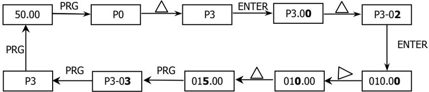
In level 3 menu, if there is no flashing bit, it indicates that the function code cannot be modified. The possible reasons include:
