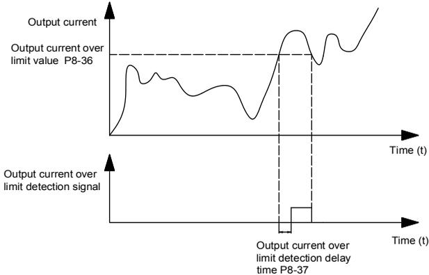
Figure 6-21 Output current over limit function diagram
