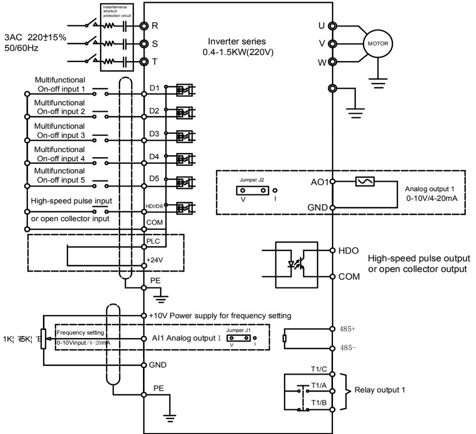
Figure 3-3 Wiring Diagram (0.4~1.5kW)
