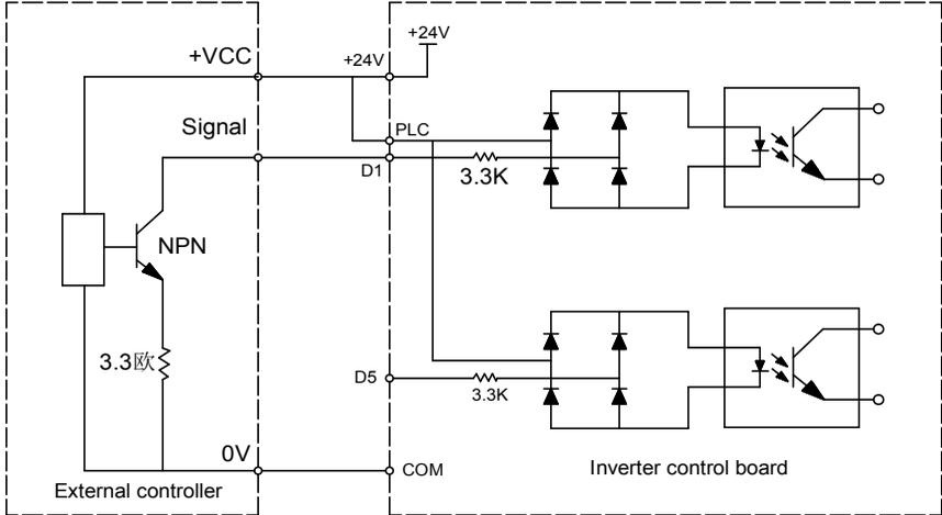
Figure 3-8 Drain wiring
