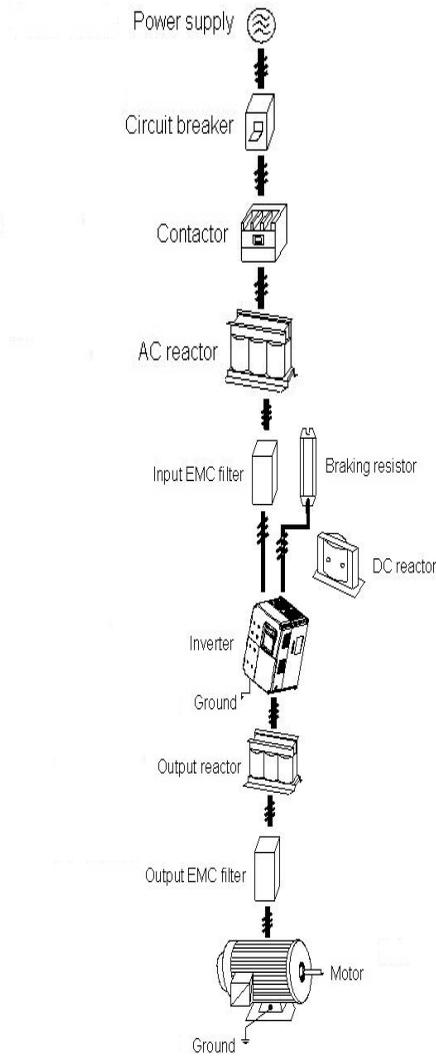
Figure3-2 Diagram of the connection to peripheral devices
