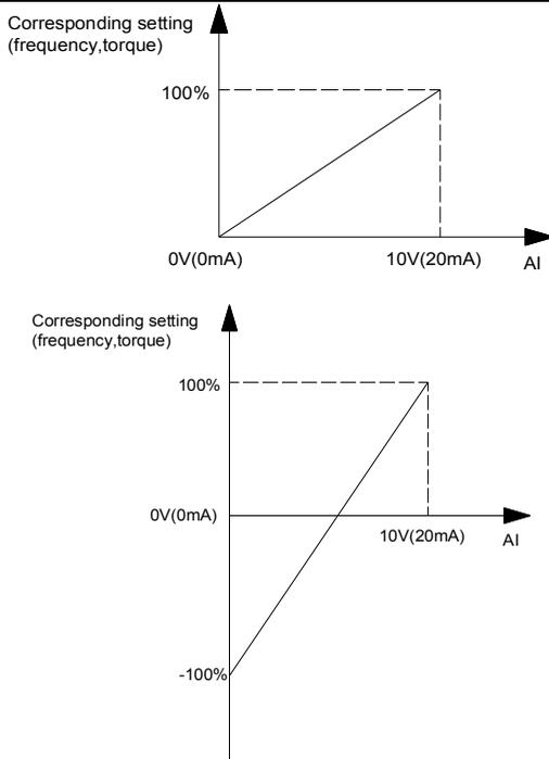
Figure 6-9 Corresponding Relationship between Analog Reference and Setting
