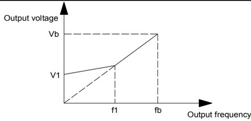
V1:Manual torque boost voltage    Vb:Maximum output voltage
