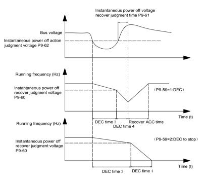
Figure 6-23 Instantaneous stop action diagram
