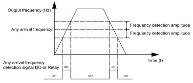
Figure 6-19 Any arrival frequency detection diagram
