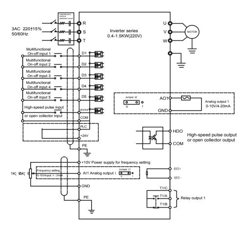
Figure 3-3 Wiring Diagram (0.4~1.5kW)
