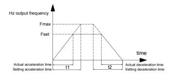
Figure 6-1 ACC/DEC time diagram
