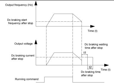
Figure 6-12 DC braking diagram
