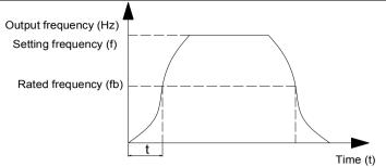
Figure 6-11 S-curve ACC/DEC A diagram
