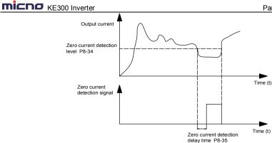
Figure 6-20 Zero-current detection diagram
