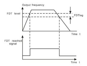
Figure 6-15 FDT Level and lag diagram
