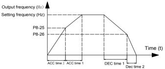
Figure 6-18 ACC/DEC time switching diagram
