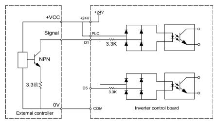
Figure 3-8 Drain wiring
