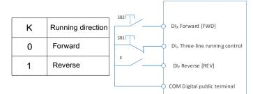
Figure 6-8 Three-line Running Mode 2
