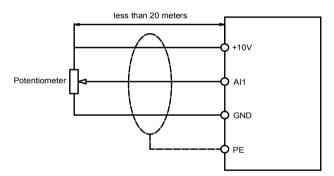
Figure 3-6 Connection of analog input
