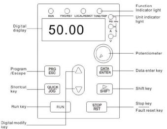
Figure4-1 Operation Keypad Diagram
