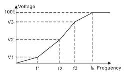
Figure 6-4 V/F curve setting diagram
