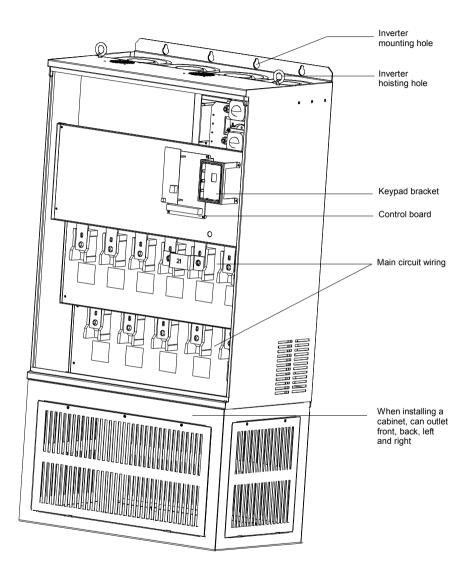
Figure 2-3 Parts of inverter
