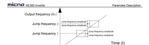
Figure 6-13 Jump frequency diagram
