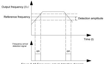
Figure 6-16 Frequency arrival detection diagram
