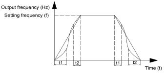
Figure 6-10 S curve ACC/DEC diagram
