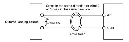
Figure 3-7 Connection of analog Input
