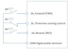
Figure 6-7 Three-line Running Mode 1
