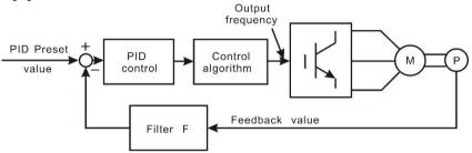
Figure 6-24 PID control diagram
