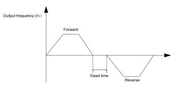
Figure 6-14 FWD/REV dead time diagram
