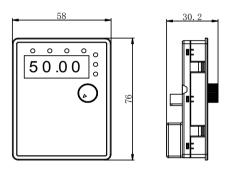
Keypad dimension of 1AC/3AC 220V 0.4~1.5kW inverter
