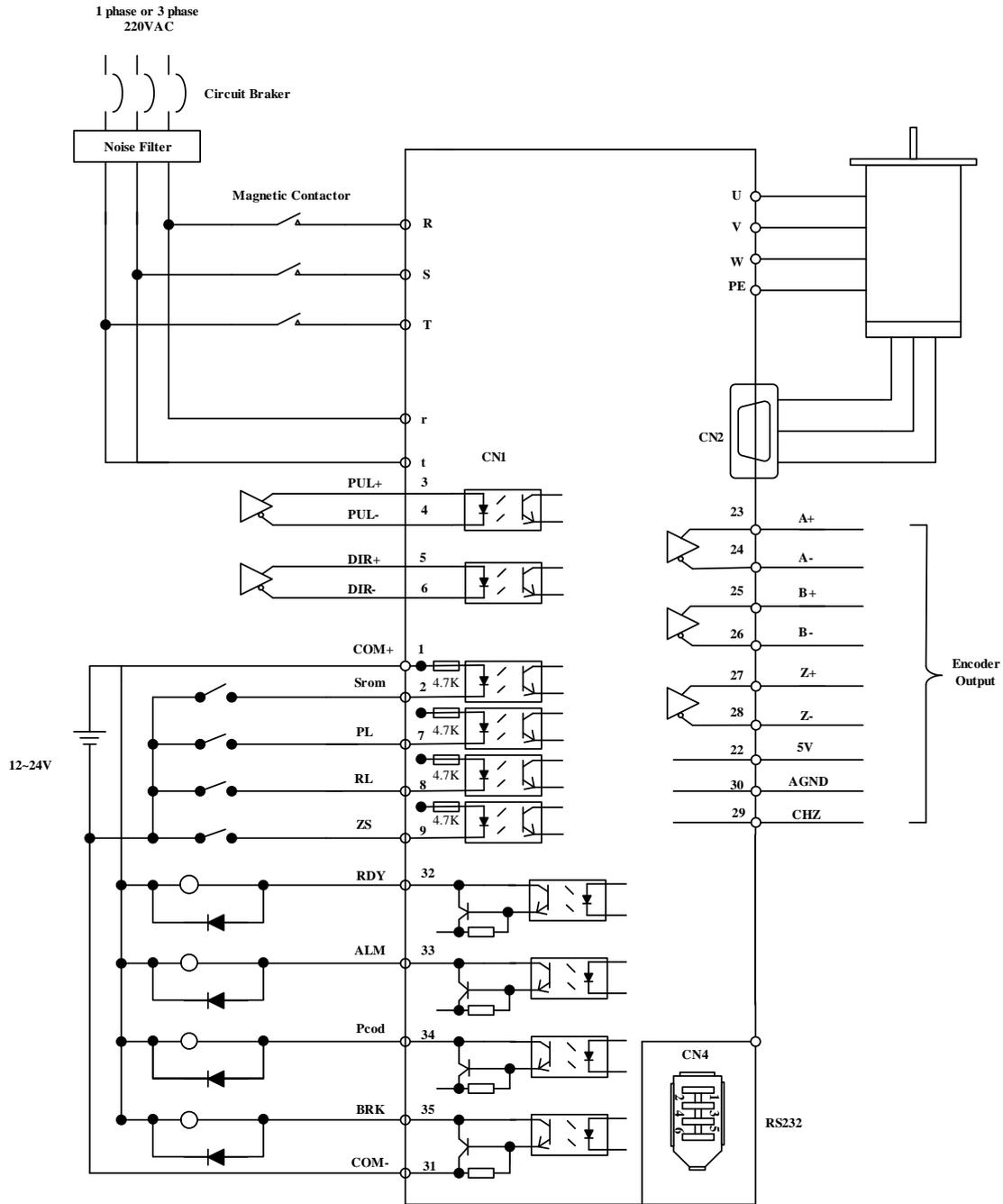
Figure 3-1 Positional Control Mode Wiring
