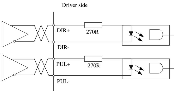
**Figure 3-6 Pulse Input Interface Differential Drive Mode**
