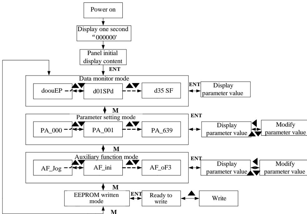
Figure 6-2 the flow diagram of panel operation
