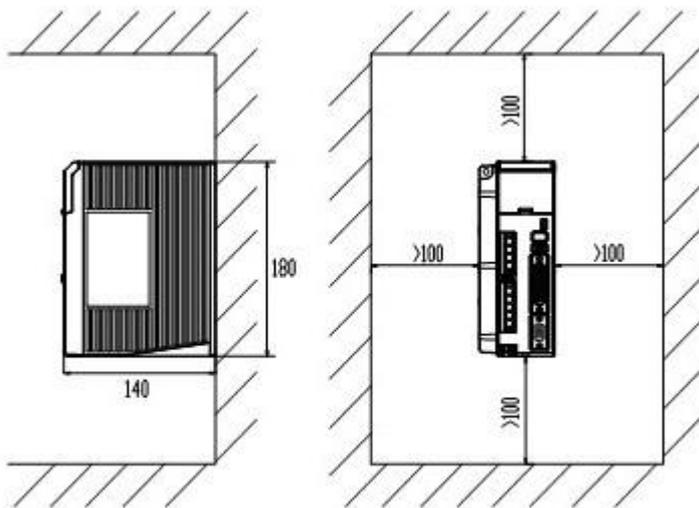
Figure 2-4 Installation Space for Single Driver
