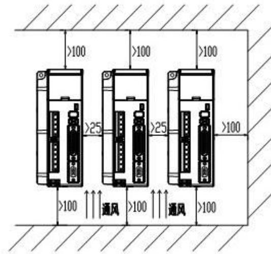
Figure 2-5 Installation Space for several Drivers
