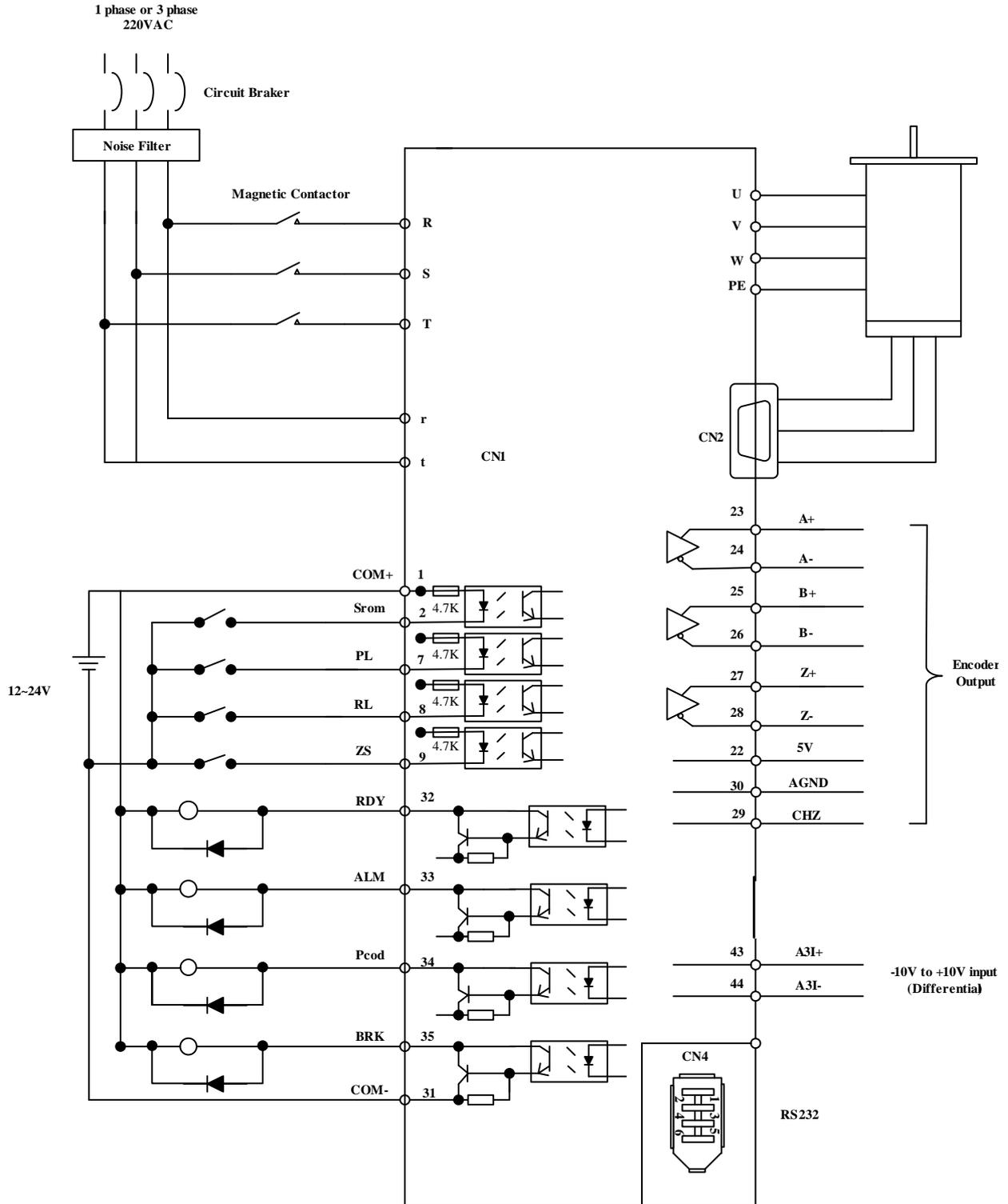
Figure 7-8 Torque Mode Typical External Wiring Diagram
