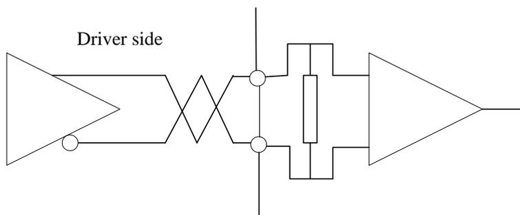
Figure 3-11 Servo Motor optical-electrical Encoder Input Interface
