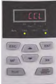
Fig. 4-4 Fault alarm display status (CCL: coder disconnection fault)
