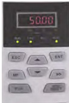
Fig. 4-3 Running parameter display status (Displaying running frequency – 50.00Hz)
