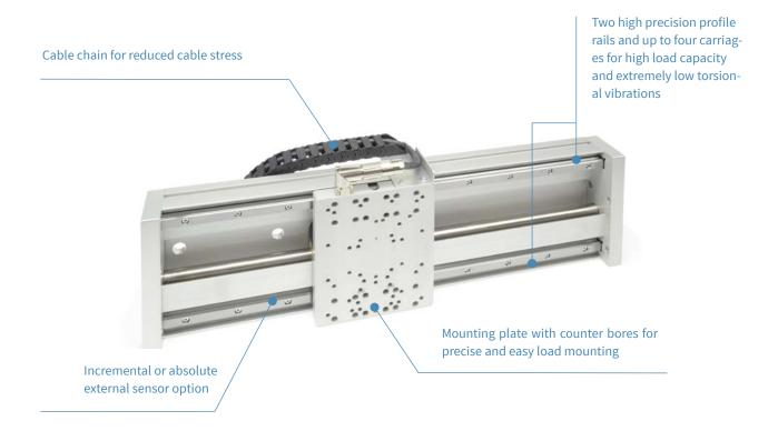
Our moving stator linear modules & guides offer a high guidance accuracy, a precise load positioning and a reliable operation even with heavy loads and over a long distance. They consist of a special aluminium profile on which up to 2 high precision rails with up to 4 linear ball bearing carriages can be mounted.
