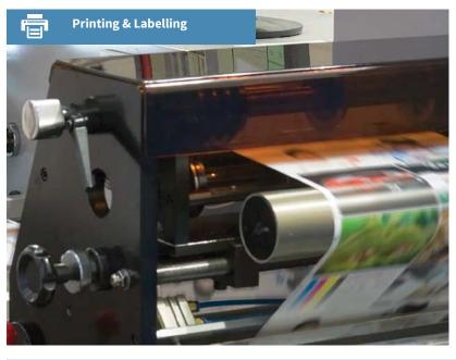
Sensitive products can be printed more quickly using linear motor technology, because the printing process is performed using position, speed, and force control. The force impacts associated with pneumatic solutions do not occur.
