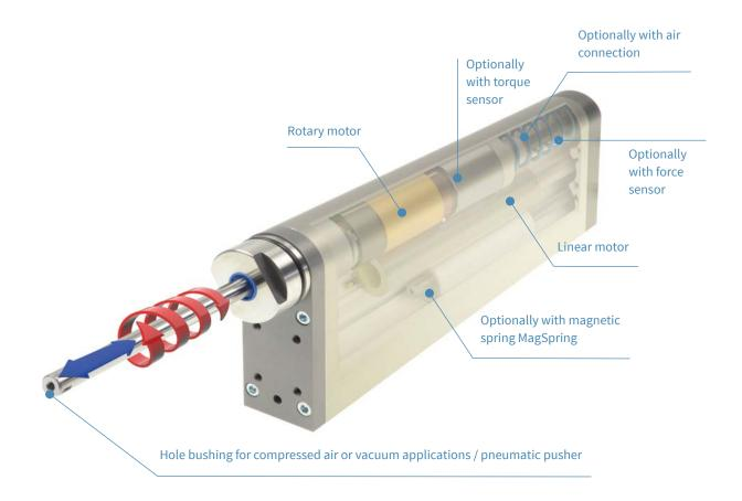
The PR02 motor series is characterized by a design wherein the motors and additional components are integrated in a slim easy to clean housing. Options can be installed such as a hollow shaft, pneumatic pusher, a magnetic spring "Mag-Spring", a torque sensor, and a force sensor.
