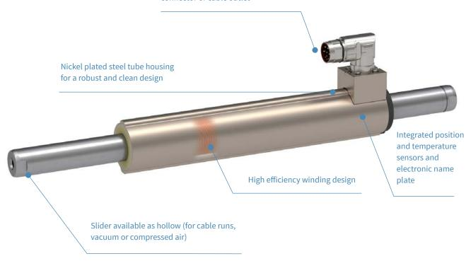
LinMot P01 linear motors are permanently actuated ironless synchronous servo motors with integrated position measurement and over-load protection. Powerful rare-earth magnets in the slider and windings in the stator are used to directly generate the linear motion.
