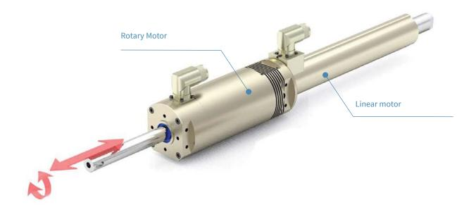
The PR01 product family combines a linear and a rotary motor in just one housing. The two electromagnetic servo motors are built in series and thus enable the installation of this machine element in the smallest possible footprint. Numerous options such as the MagSpring load compensation, pneumatic brake, cam kit and wiper can be added to the module.
