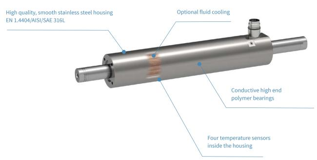
In a surrounding where explosive gases, vapor-air mixture or combustible dust can form, special electric motors are required. LinMot ATEX has been developed exactly for those special conditions. The motors are built with the awareness to operate in an explosive environment. For this, the stator is completely encapsulated with epoxy resin and an additional temperature monitoring is integrated into the motor as the surface temperature is of crucial importance in an explosive atmosphere.
