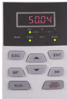
Fig. 4-7 Direct frequency modification status
