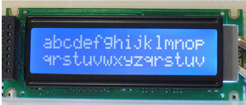
Figure 21: Typical 2x16 character LCD
