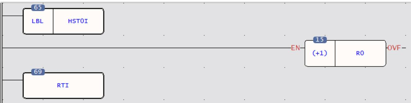
Figure 9 The interrupt sub-program example of cyclic pulse
