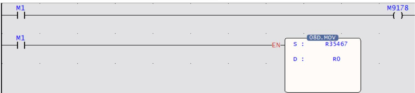
When M1=1, M9178 HSTA cycle timer control is triggered, and the value in the special register DR35467 is moved into R0.
