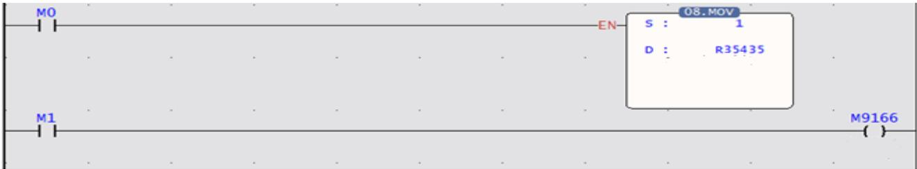
When M0=1, set the interrupt cycle of STM0 as 1ms. After R35435=1 and M1=1, the STM0 will execute timing interrupt once every 1ms.
